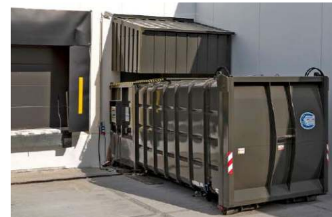
Left: Eco-compactor in the receiving area of the Moniga del Garda branch
