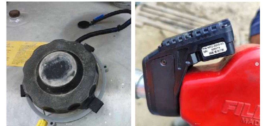
Left: RFID tag. Right: Gun Reader Read vehicle ID data and transmit an RF signal to the RFID communication antenna to initiate the refuelling process and stop it when it finishes. www.controlims.com/fleetcontrol/
